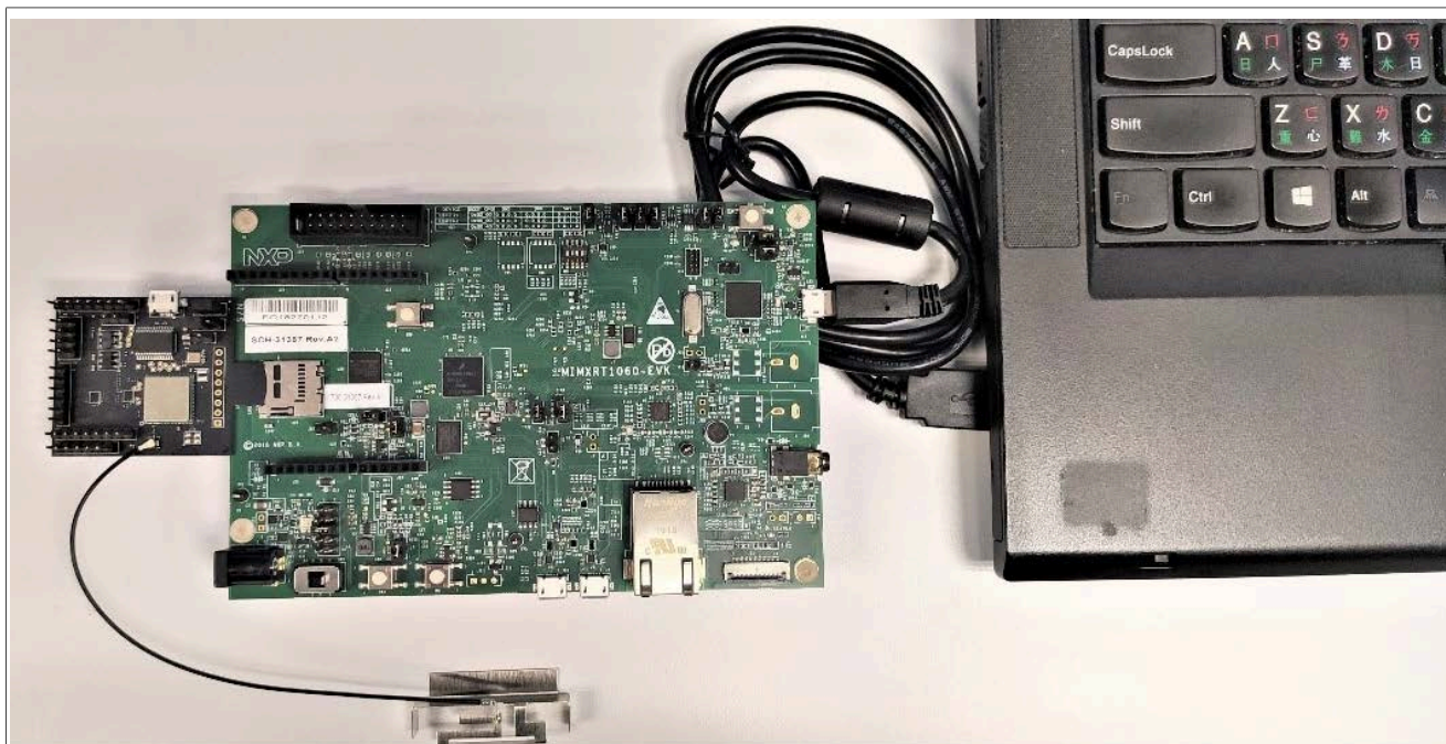
Figure 12. i.MX RT1060 EVK board connection to host computer for power supply and console access
