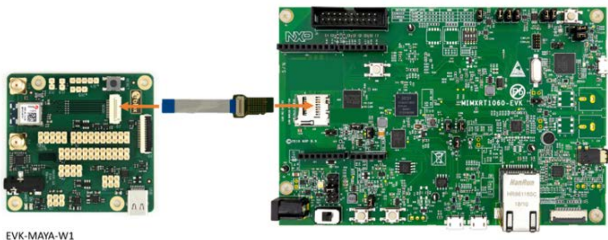
Figure 15. : u-blox EVK-MAYA-W1 connected to i.MX RT1060 EVK using uSD interface
