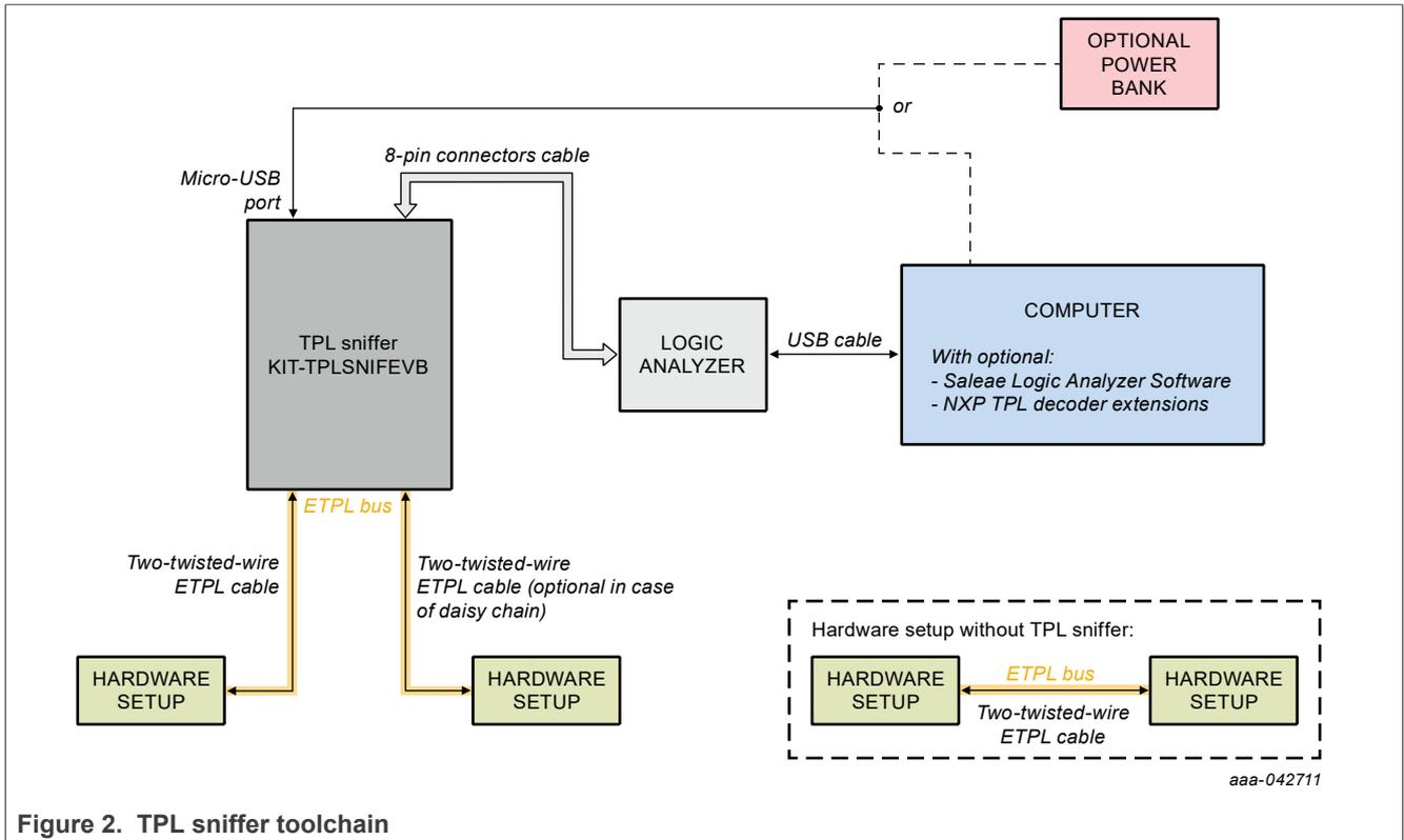
Figure 2. TPL sniffer toolchain
