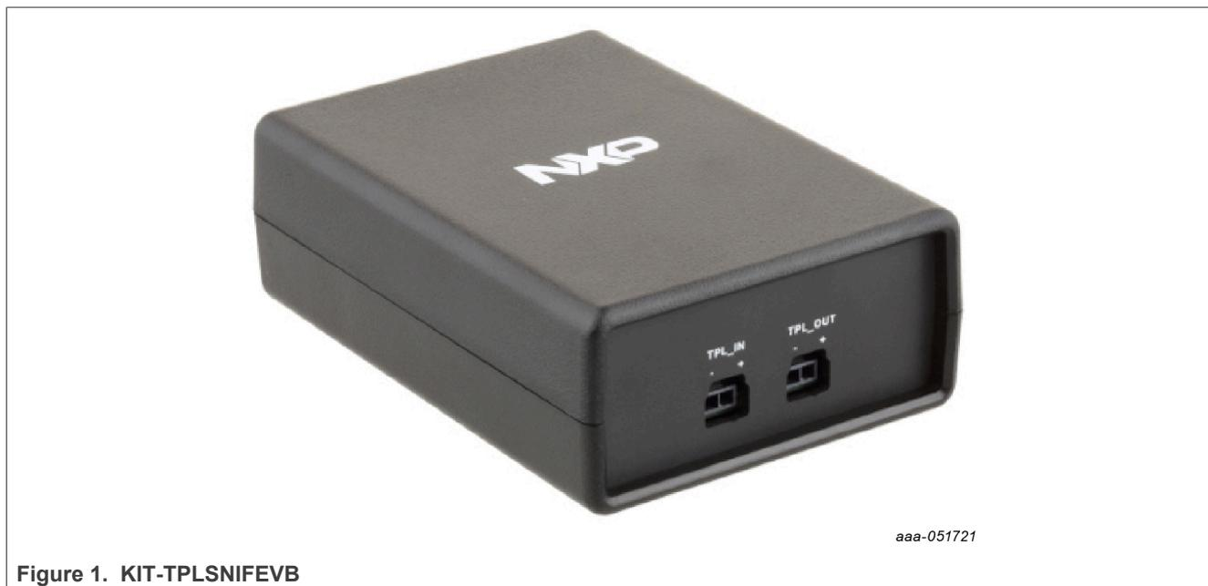
Placed in any ETPL bus, it non-intrusively listens to all messages and monitors the frame traffic on the bus (the TPL sniffer works in listen mode only). The corresponding received data [in serial peripheral interface (SPI) format] is available on the analyzer output connector (see [Figure 6](#)), to be connected to a logic analyzer and its software which provides further analysis of such data.
