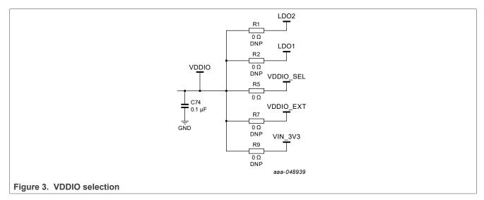
The I<sup>2</sup>C is compatible with 1.8 V, 3.3 V, and 5.0 V, therefore VDDIO\_SEL voltage is configurable between 1.8 V, 3.3 V, or 5.0 V using SJ8, SJ9, and SJ10 connectors (3.3 V by default) shown in Figure 4.
