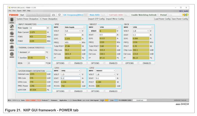
VPRE external MOSFET parameters can be added on the VPRE > OPTIONS > EXTERNAL MOSFET SELECTION option and then chosen with VPRE > OPTIONS > COMPONENT SELECTION. Special care must be given to MOSFET thermal resistance.
