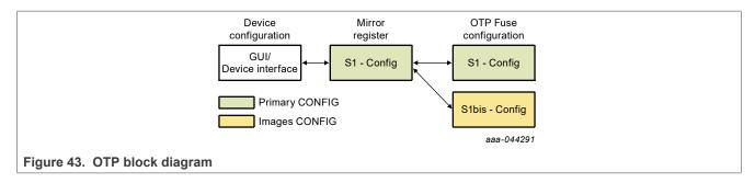
At device starts-up, the content of the valid (last programmed) sector is loaded into mirror registers. The mirror register content is accessible from the NXP GUI, using specific I<sup>2</sup>C commands. The NXP GUI manages the mirror configuration, which facilitates access. The mirror register content handling is called "OTP emulation".
