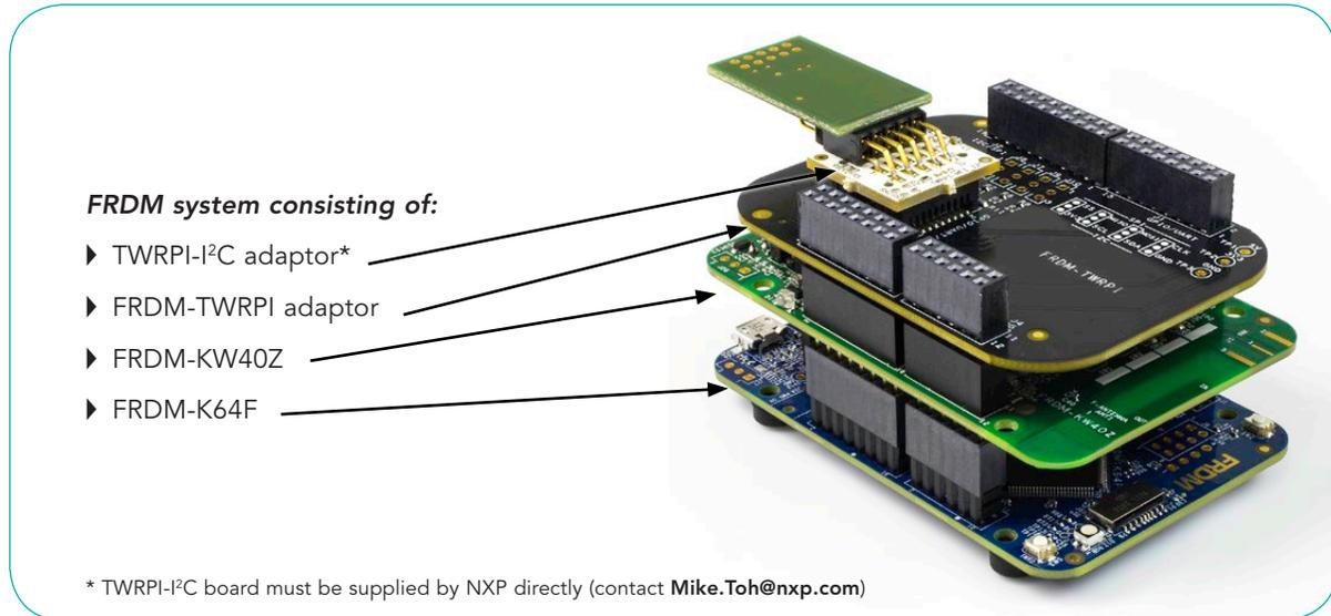
The low-cost NXP Freedom development board platform is supported with the HomeKit software for easy evaluation, development, and rapid prototyping. Additional hardware details can be found in the SDK's documentation and release notes.
