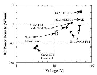
Fig.4. RF power density vs. voltage for GaAs FET's, Si LDMOS FET's, GaN FET, and 4H-SiC FET.
