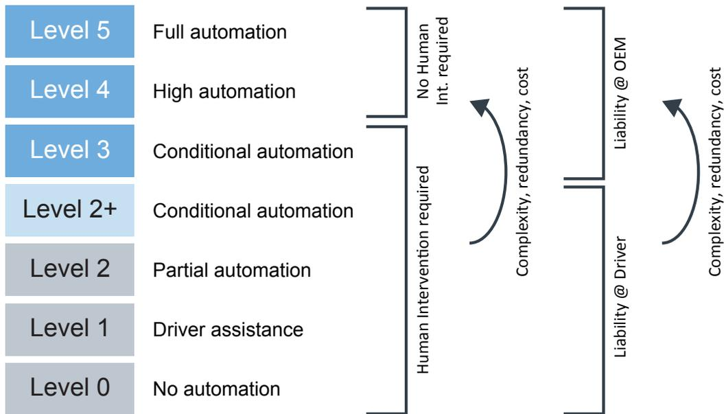
Figure 1: Levels of Advanced Driving Assistance Systems and Autonomous Driving
