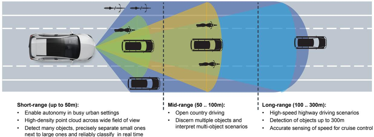
Figure 3: Simultaneous triple beam multi-mode for short-, mid- and long-range capability
