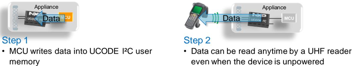
**Figure 5 Zero-power read process using the UCODE I<sup>2</sup>C dual-interface memory. Here the read process with a hand-held UHF reader is shown.**
