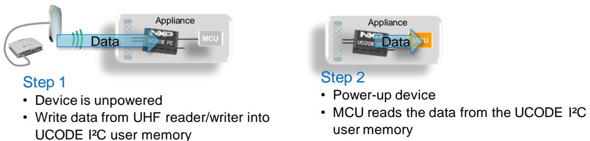
**Figure 4 Zero-power write process, using the UCODE I<sup>2</sup>C dual-interface memory. Here the write process with a stationary UHF reader plus antenna is shown.**
