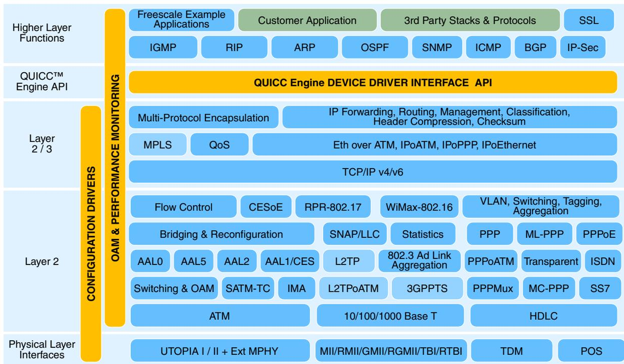
Figure 3. Software Protocol Support for the QUICC Engine
