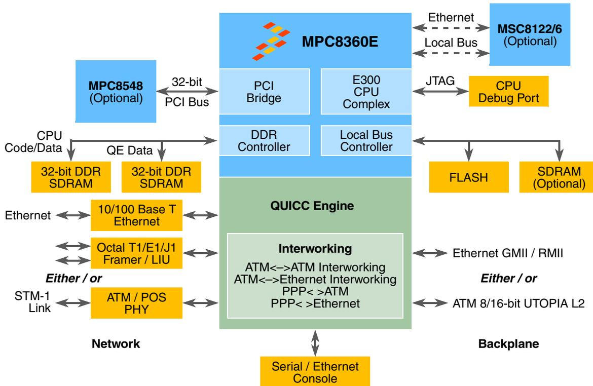
Figure 4. NodeB Network Interface Card Using the MPC8360E
