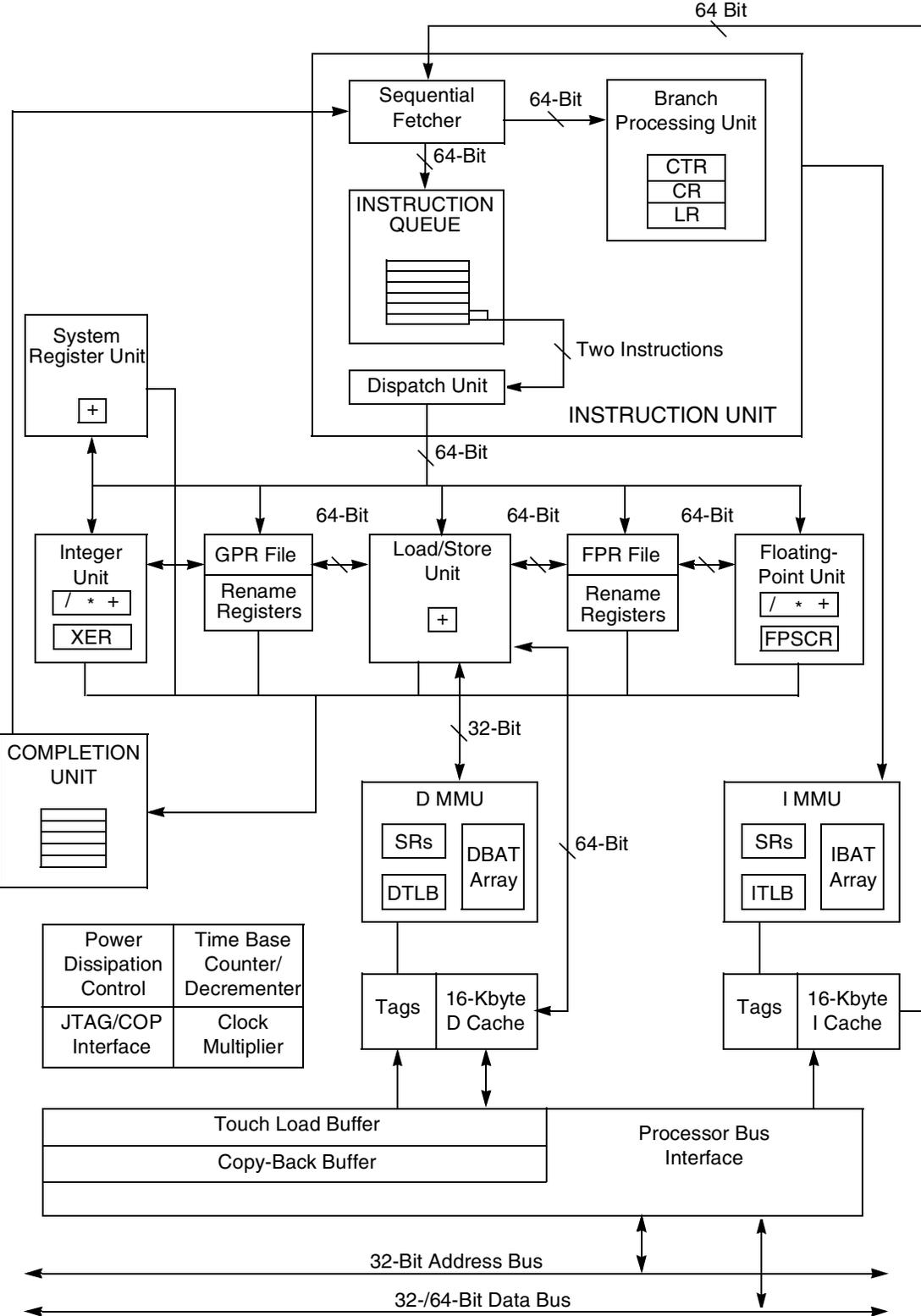
Figure 1. MPC603 Block Diagram
