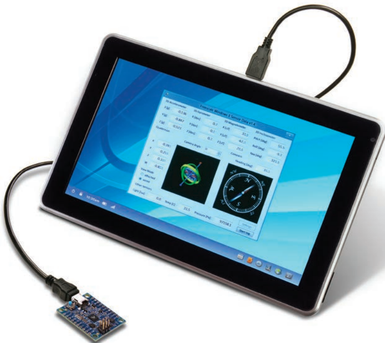
Figure 4. The display/user interface for the gyroscope and magnetometer in the sensor reference platform on a tablet running Microsoft Windows 8.
