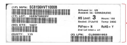
MBB label for material tested at KLM Test
