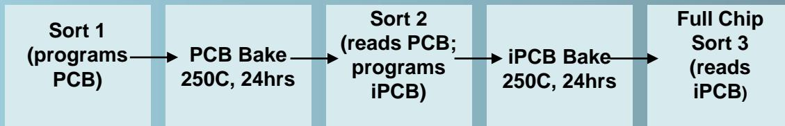
The current flow utilizes the Physical/Inverse CheckerBoard (PCB/iPCB) patterns in 2 inserts.
