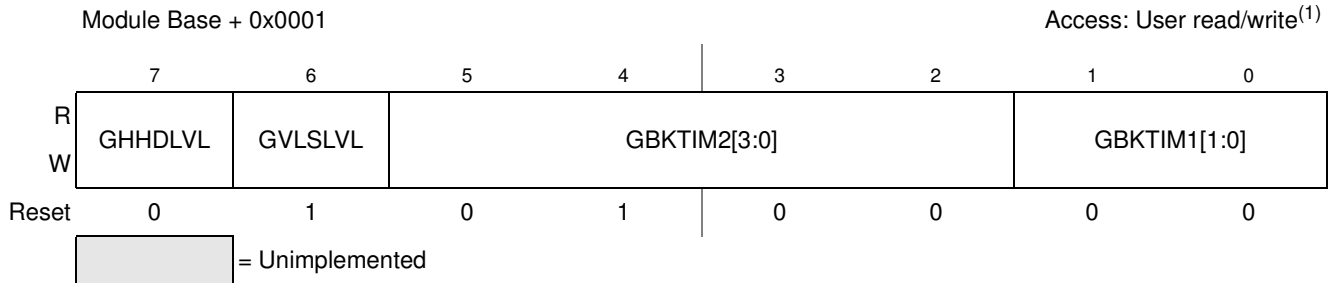
Figure 17-4. GDU Control Register (GDUCTR)
