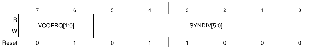
Figure 8-5. S12CPMU_UHV_V6 Synthesizer Register (CPMUSYNR)
