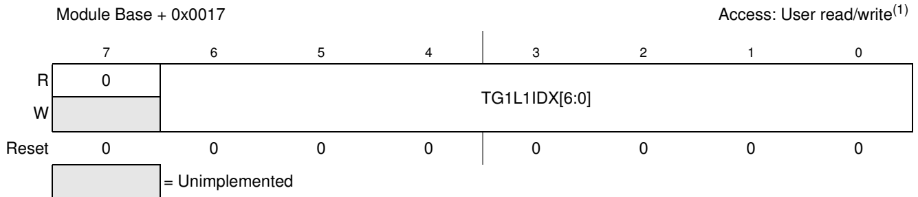
Figure 13-20. Trigger Generator 1 List 1 Index (TG1L1IDX)
