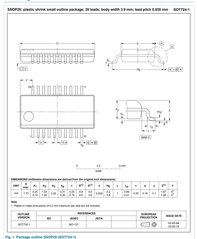
plastic shrink small outline package; 20 leads; body width 3.9 mm; lead pitch 0.635 mm
