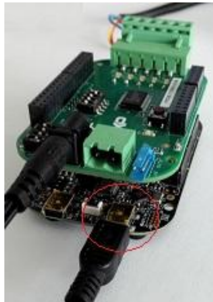
Figure 3 OpenSDA PC-MCU Debug Connection
