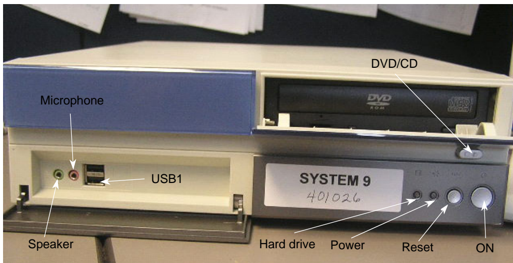
Figure 2. Front of Box with Open Door
