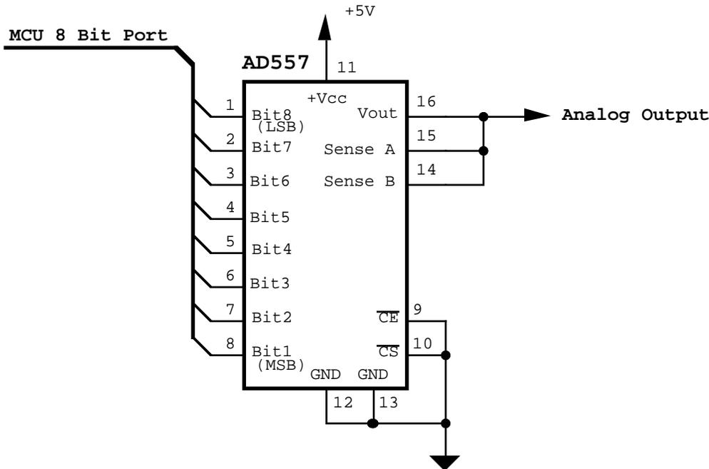
**Figure #1 - Basic schematic for the AD577 Digital-to-Analog Converter**
