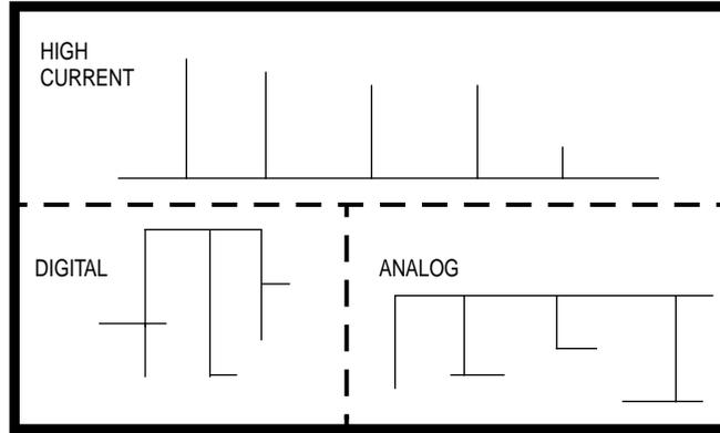
**Figure 5. Separation of Circuits on a PCB**
