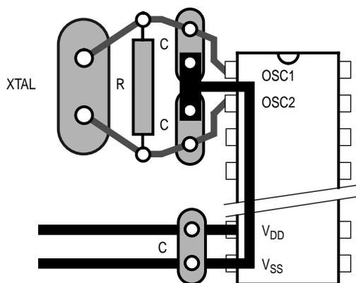
**Figure 11. Crystal or Ceramic Resonator Circuit Layout**
