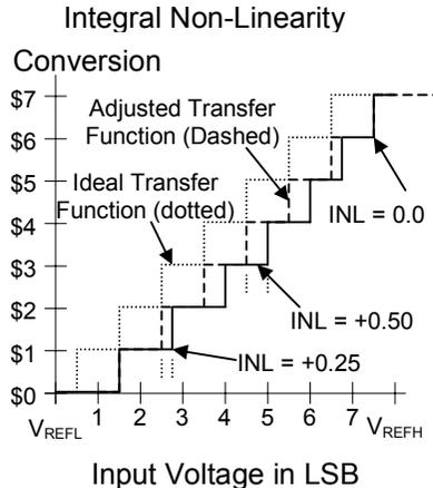
*Integral Non-Linearity (INL)* is defined as the sum from the first to the current conversion (integral) of the non-linearity at each code (*Code DNL*). For example, if the sum of the DNL up to a particular point is 1LSB, it means the total of the code widths to that point is 1LSB greater than the sum of the ideal code widths. Therefore, the current point will convert one code lower than the ideal conversion.
