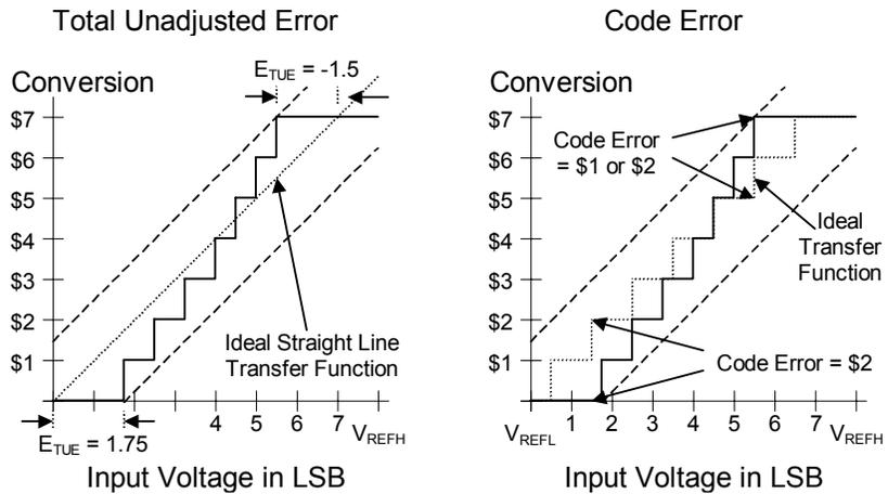
**Figure 4. Total Unadjusted and Code Error Graphs**
