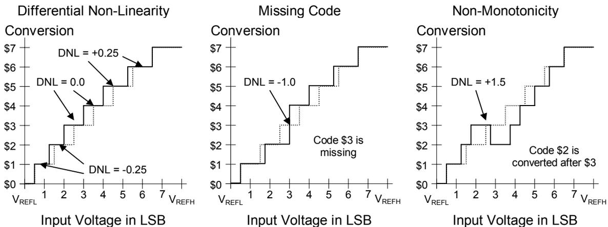
Figure 3. Differential Non-Linearity, Missing Codes, and Non-Monotonicity Graphs
