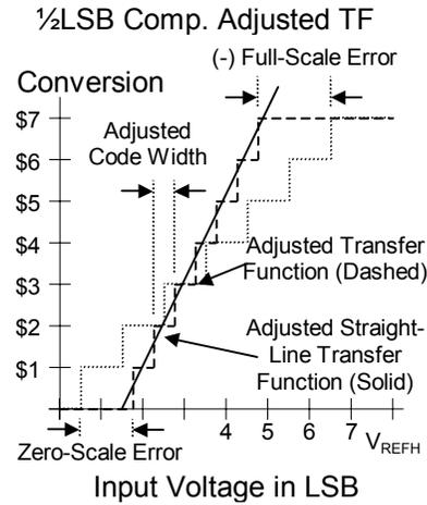
Most ADC's exhibit some non-linearity at the endpoints due to the difficulty in measuring a signal that is identical to the reference. If these errors are accounted for, a more accurate portrayal of the ADC behavior in application is possible. For this reason, the *Adjusted Straight-Line Transfer Function* is drawn between the minimum input voltage plus the *Zero-Scale Error* ( $V_{REFL} + E_{ZS}$ ) to the maximum input voltage plus the *Full-Scale Error* ( $V_{REFH} + E_{FS}$ ).
