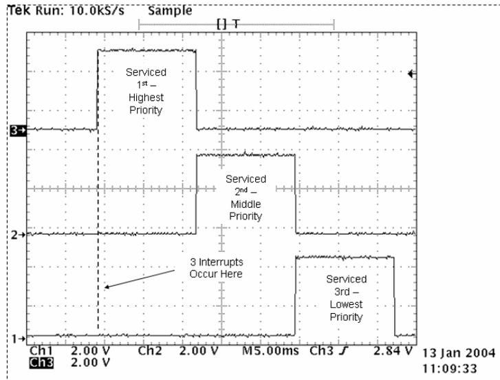
Figure 6. Interrupt Priority Execution — Simultaneous Occurrence of Interrupts
