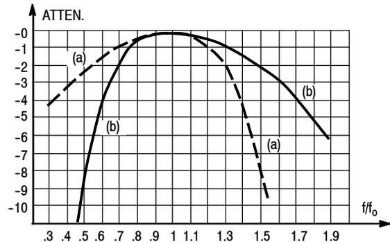
Figure 14. Selectivity Curves for Networks (a) and (b) of Figure 13
