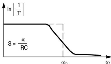
**Figure 22. Representation of Bode Equation**
