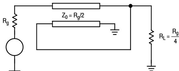
**Figure 28. 4:1 Line Transformer**
