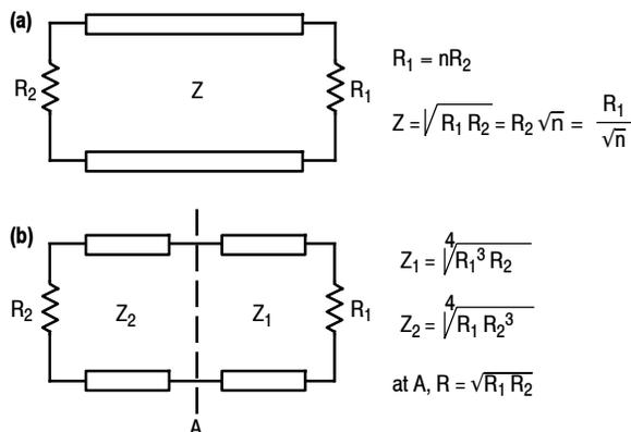
**Figure 18. Transformation Networks Using  $\lambda/4$ -Long Transmission Lines**
