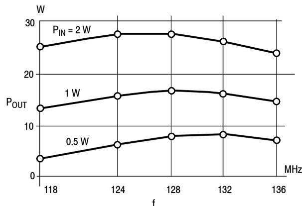
**Figure 38. P<sub>OUT</sub> vs Frequency**
