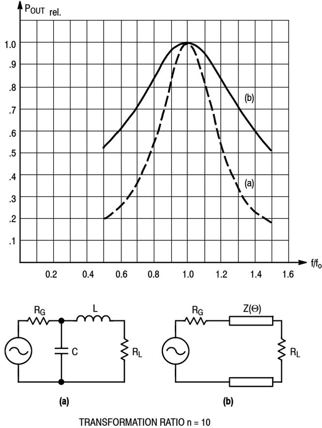
**Figure 8. Bandwidth of the L-Section for  $n = 10$**
