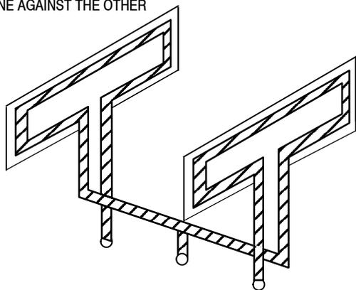
**Figure 29. 4:1 Line Transformer on P.C. Board**
