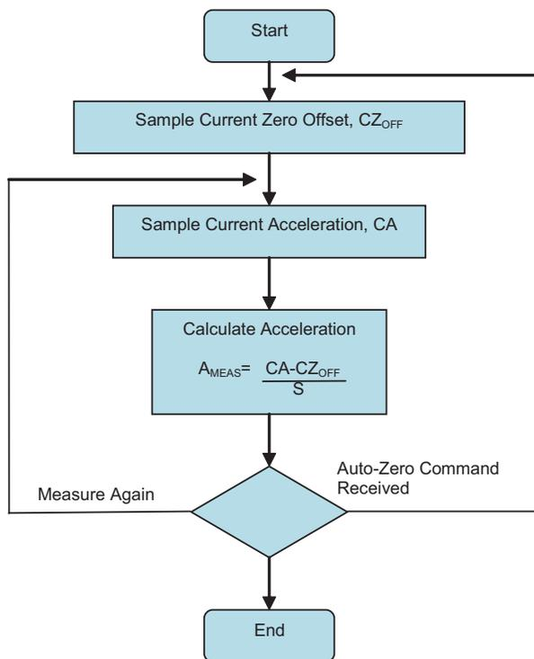
Figure 3. Flow Chart of the Auto-Zero Algorithm
