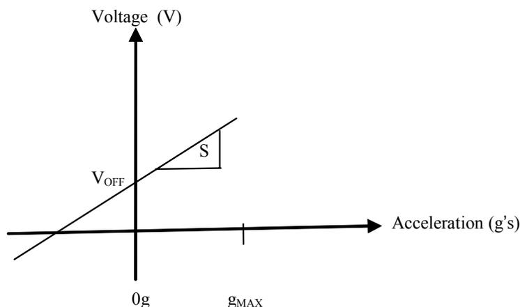
**Figure 1. Transfer Function of the Accelerometer Sensor**
