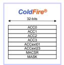
The Enhanced Multiply-Accumulator (eMAC) unit can be found on most V2, on V3, and on V4 cores. eMAC is faster and more accurate for math-intensive software algorithms, such as optimizing audio decoding/encoding for MP3. The eMAC features four 48-bit accumulators. The eMAC allows for 16x16 and 32x32 multiplies with a 40-bit product.
