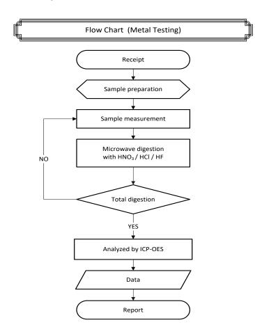
\*\* Remarks : The samples were dissolved totally by pre-conditioning method according to above flow chart.
