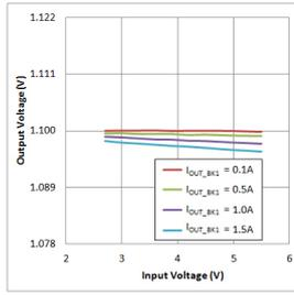
Figure 30. Buck1 output voltage vs input voltage WLCSP-12
