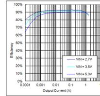
Figure 23. Buck2 (2.2V) efficiency vs output current WLCSP-12
