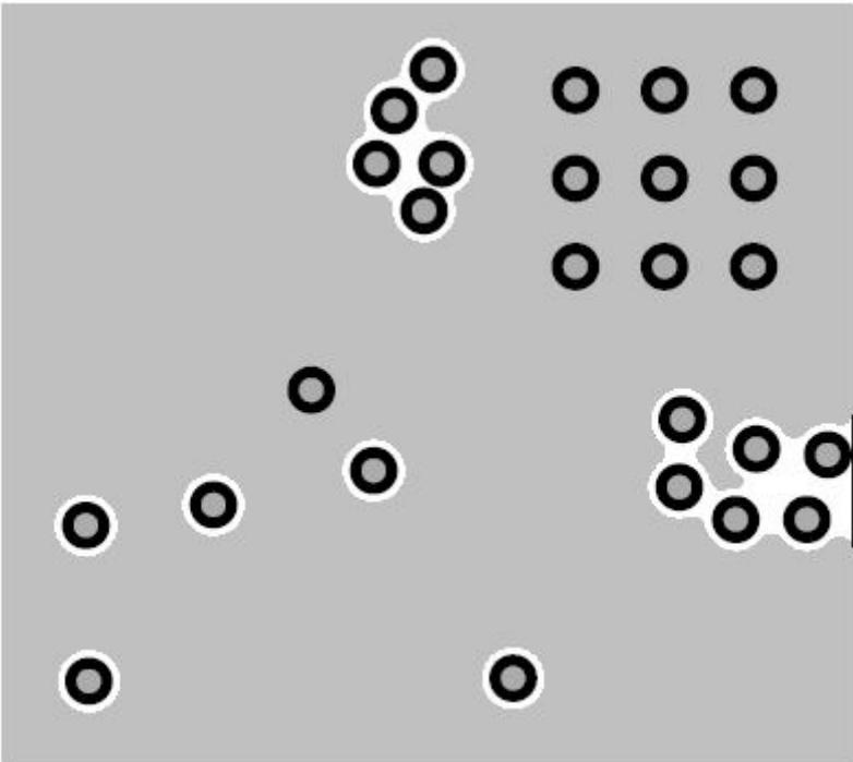
Figure 56. Layer 3 vias and copper (not to scale)
