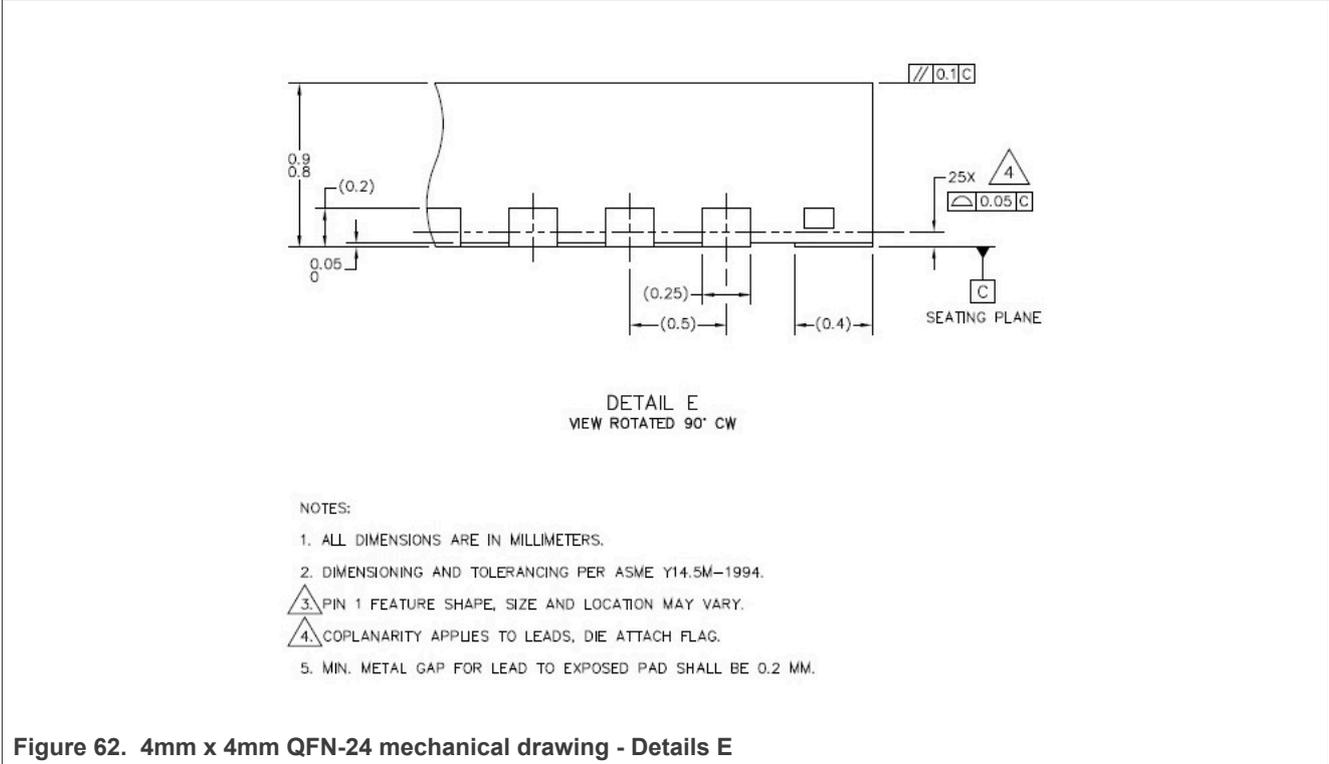
Figure 62. 4mm x 4mm QFN-24 mechanical drawing - Details E
