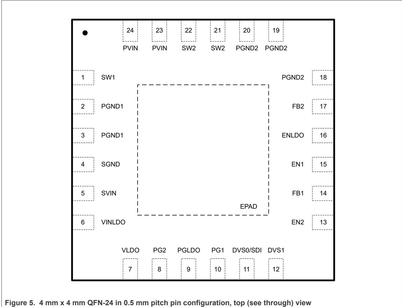
Figure 5. 4 mm x 4 mm QFN-24 in 0.5 mm pitch pin configuration, top (see through) view
