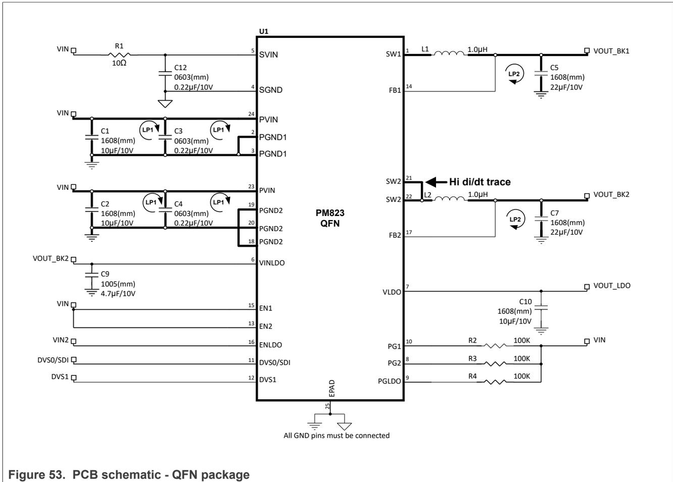
Figure 53. PCB schematic - QFN package
