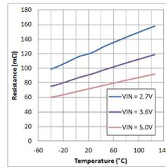
Figure 49. Buck2 high side  $R_{DS(ON)}$  vs. temperature QFN-24
