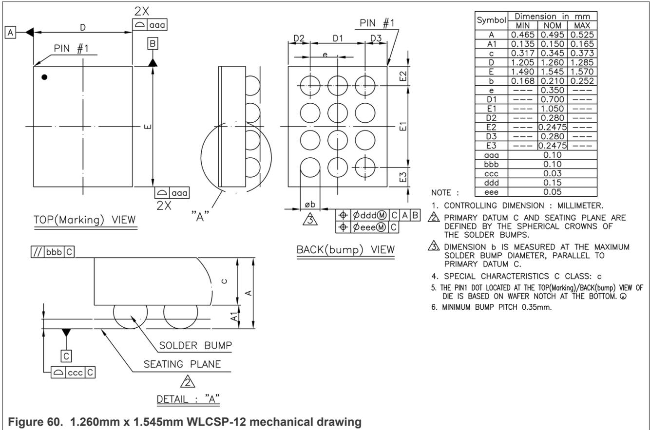
Figure 60. 1.260mm x 1.545mm WLCSP-12 mechanical drawing
