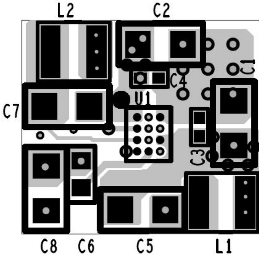
The input capacitors must be placed closely to the corresponding power and ground pins (PVIN/PGND) on the same PCB layer as the IC.
