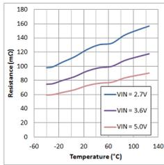
Figure 48. Buck1 high side  $R_{DS(ON)}$  vs. temperature QFN-24
