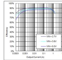
Figure 25. Buck2 (1.8V) efficiency vs output current QFN-24
