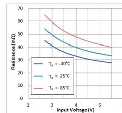
Figure 36. Buck2 low side  $R_{DS(ON)}$  vs. input voltage WLCSP-12
