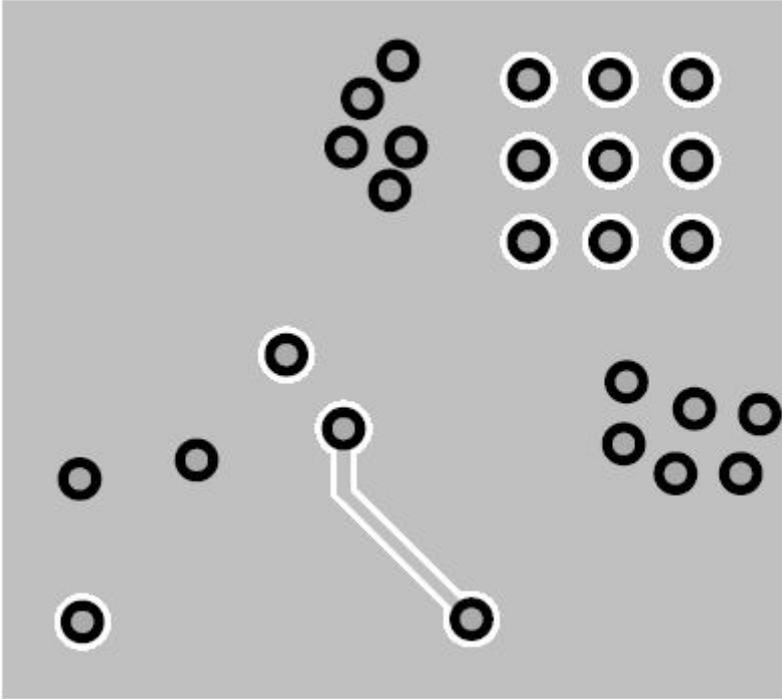
Figure 57. Bottom traces, vias, and copper (not to scale)
