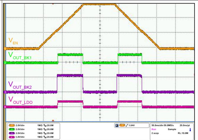
Figure 11. UVLO / OVP Thresholds
