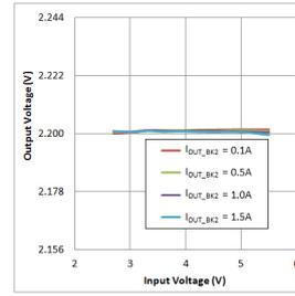
Figure 31. Buck2 Output Voltage vs Input Voltage WLCSP-12
