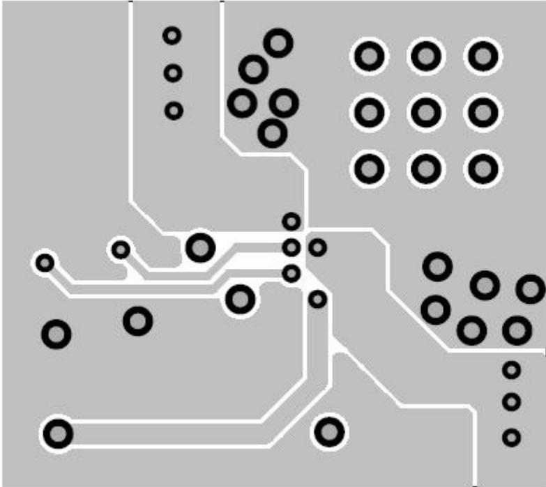
Figure 55. Layer 2 vias and copper (not to scale)
