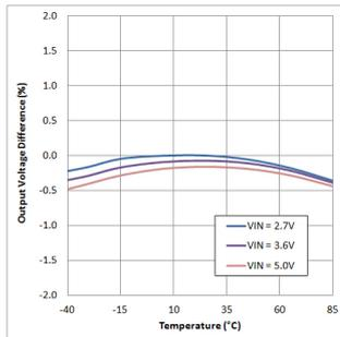
Figure 41. Buck1 Output Voltage Error vs Temperature
