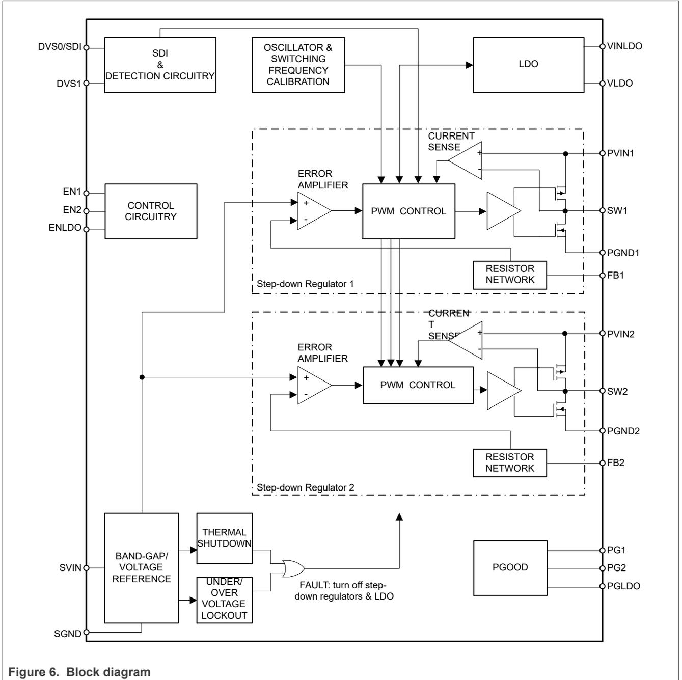
Figure 6. Block diagram
