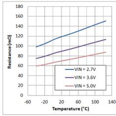
Figure 44. Buck1 high side  $R_{DS(ON)}$  vs. temperature WLCSP-12
