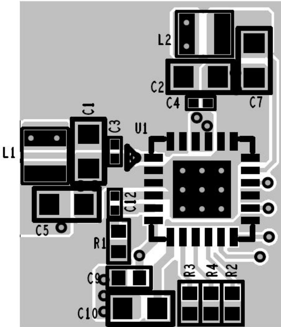
The input capacitors must be placed closely to the corresponding power and ground pins (PVIN/PGND) on the same PCB layer as the IC.
