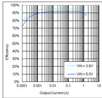
Figure 24. Buck1 (3.3V) efficiency vs output current QFN-24
