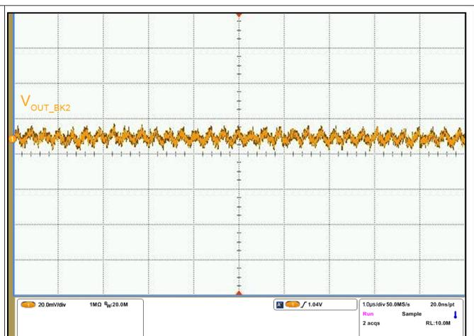
Figure 21. Buck2 (2.2V) PWM Output Ripples at 1.5A
