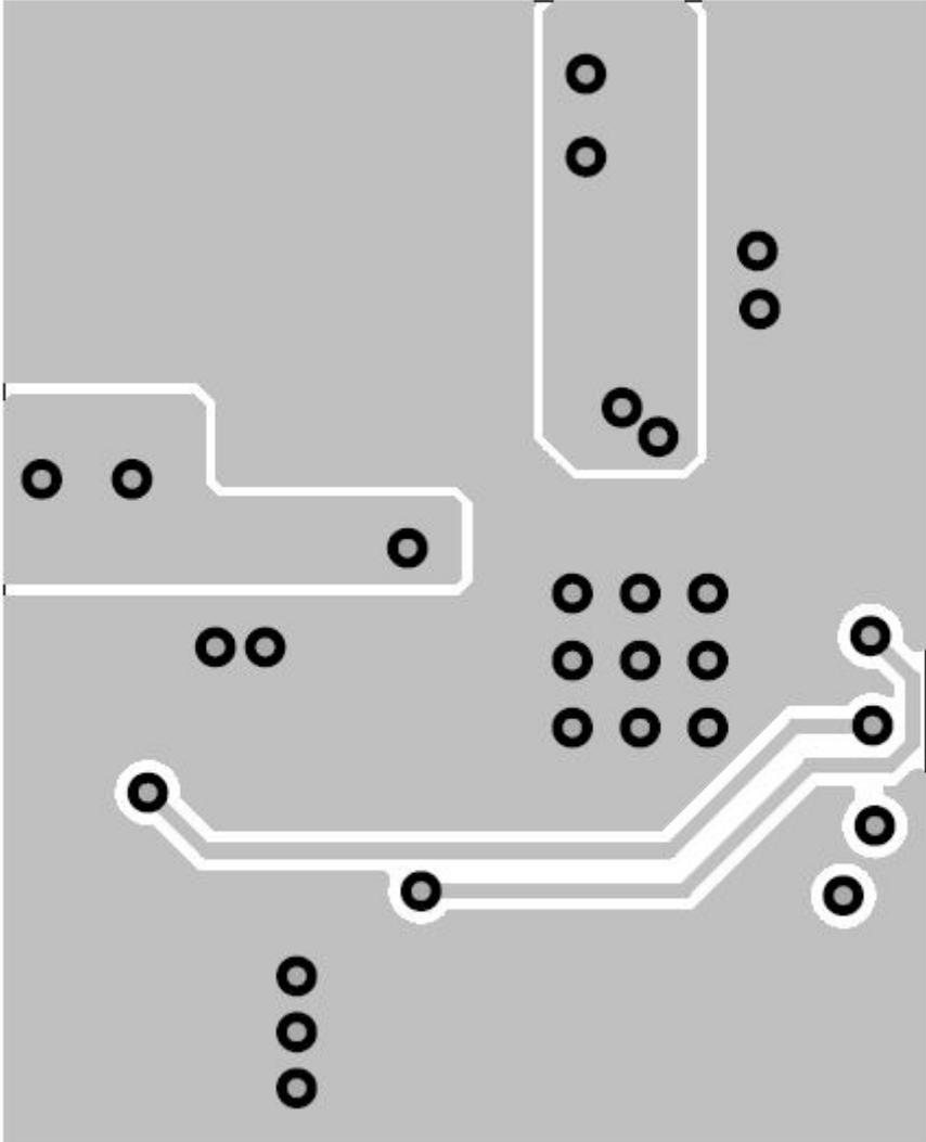
Figure 59. Bottom traces, vias, and copper (not to scale)
