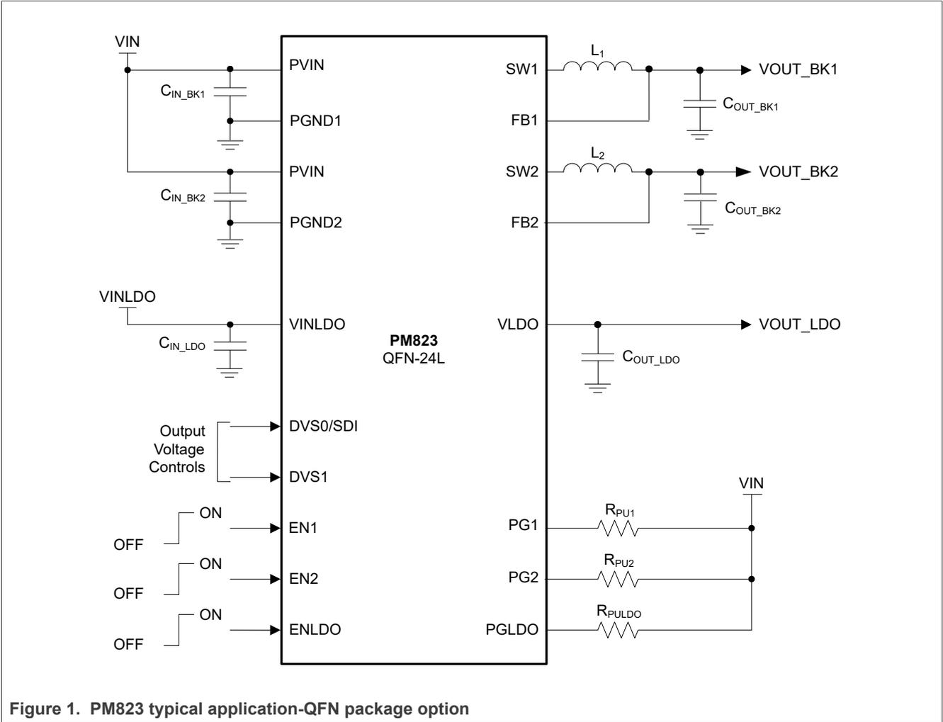
Figure 1. PM823 typical application-QFN package option
