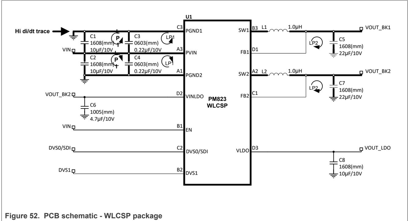
Figure 52. PCB schematic - WLCSP package
