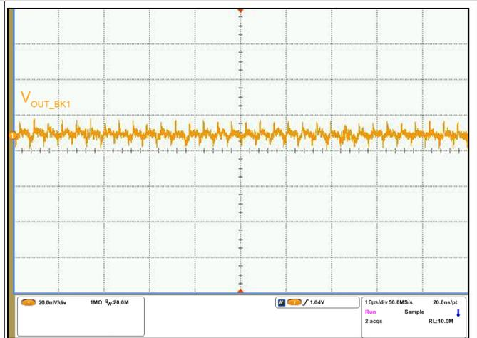
Figure 19. Buck1 (1.1V) PWM Output Ripples at 1.5A
