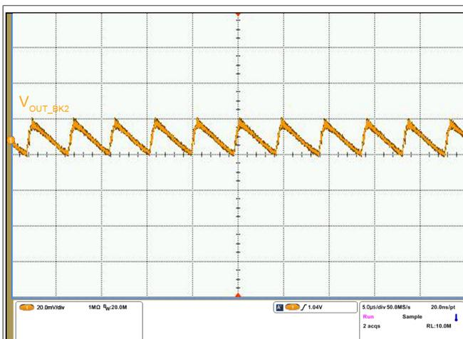
Figure 20. Buck2 (2.2V) PFM Output Ripples at 45 mA
