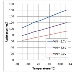
Figure 45. Buck2 high side  $R_{DS(ON)}$  vs. temperature WLCSP-12
