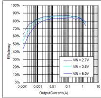
Figure 22. Buck1 (1.1V) efficiency vs output current WLCSP-12
