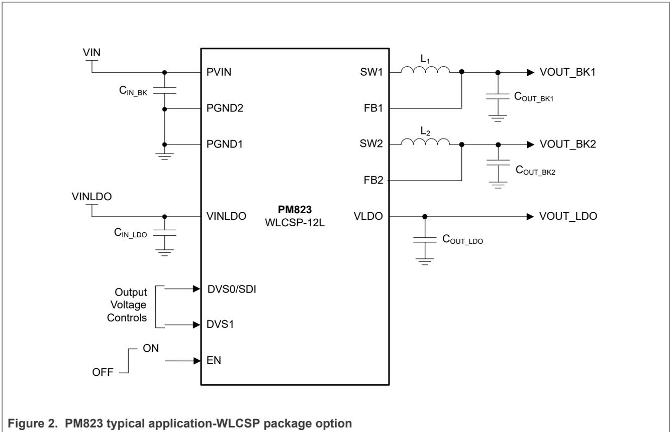
Figure 2. PM823 typical application-WLCSP package option
