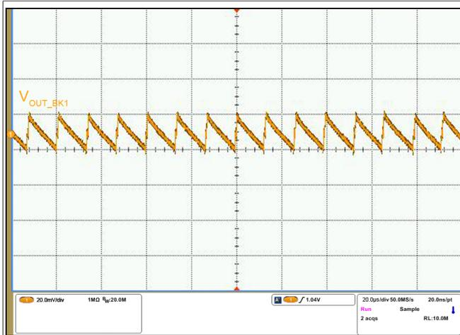
Figure 18. Buck1 (1.1V) PFM Output Ripples at 25 mA
