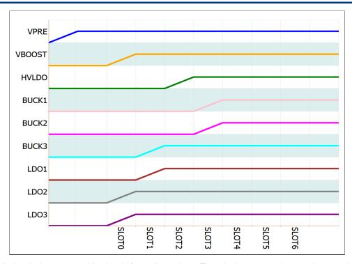
The signals depicted above are enable signals for each regulator. They don't represent the actual ramp voltage
