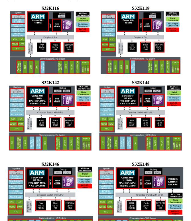
**Note:** Model-Based Design Toolbox for S32K1xx Series does not support RAM targets and peripheral that needs RAM support on S32K116, S32K118, and S32K142 microcontrollers due to the limited RAM footprint.
