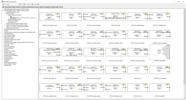
Special Simulink Blocks have been added to simplify the way a user can initialize such a controller, read vital parameters (like cell voltage, stack voltage, temperature, current) and manage the whole system. The entire suite of blocks is easily integrated within the new Battery Management Toolbox from MathWorks, so users can leverage these algorithms on top of our blocks.
